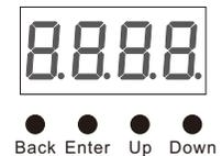
By holding button Back + Enter together at the same time over 5 seconds until the display go off, it will restore default settings .
